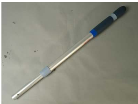
Photo 1: Telescopic Handle frame after 80 cycles
